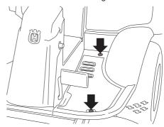
2 Loosen the locking nuts (1).
